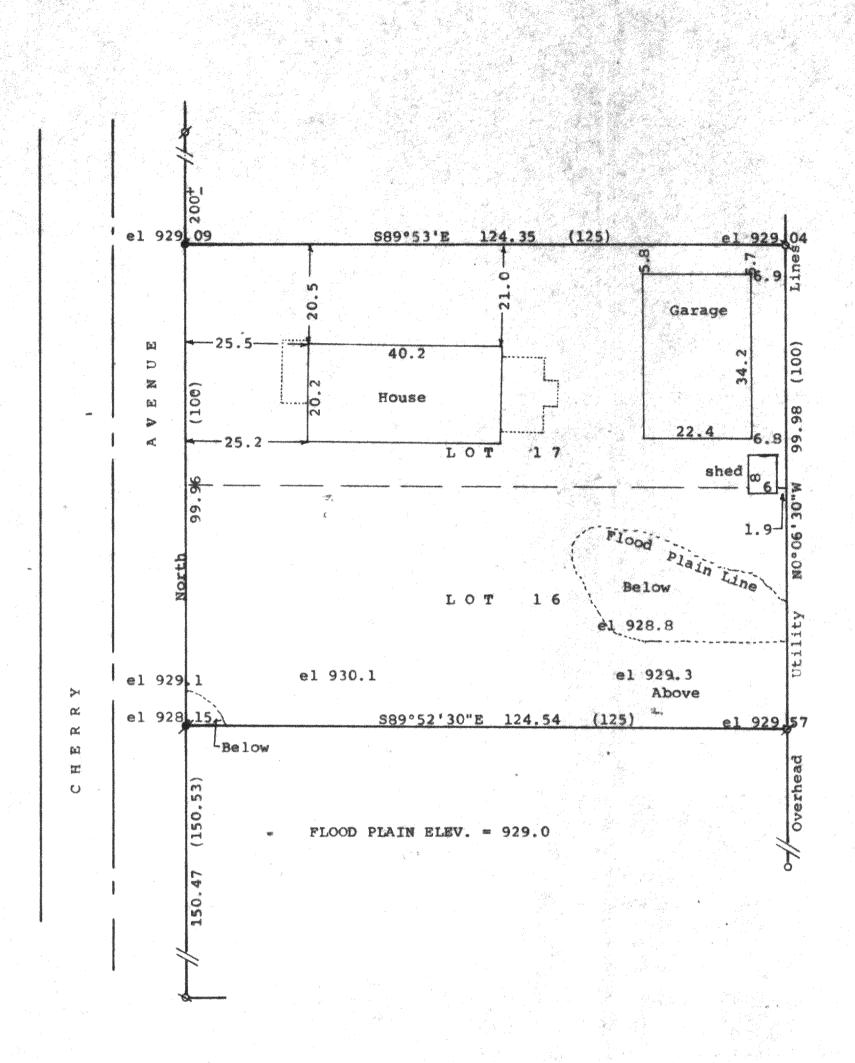
Scale - 1" = 20'  $\emptyset = 1$ ' Iron Pipe Found o = 1" Iron Pipe Found N=3/4" Iron Pipe Found # = 14" X 24" Iron Pipe Set # = 1" X 24" Iron Pipe Set (0.00) = recorded distance Bearings referenced to the east line of Cherry Avenue with the assumed bearing of North Survey ordered by: Ed Brien Lake Delavan Highlands Delavan, WI 53115
