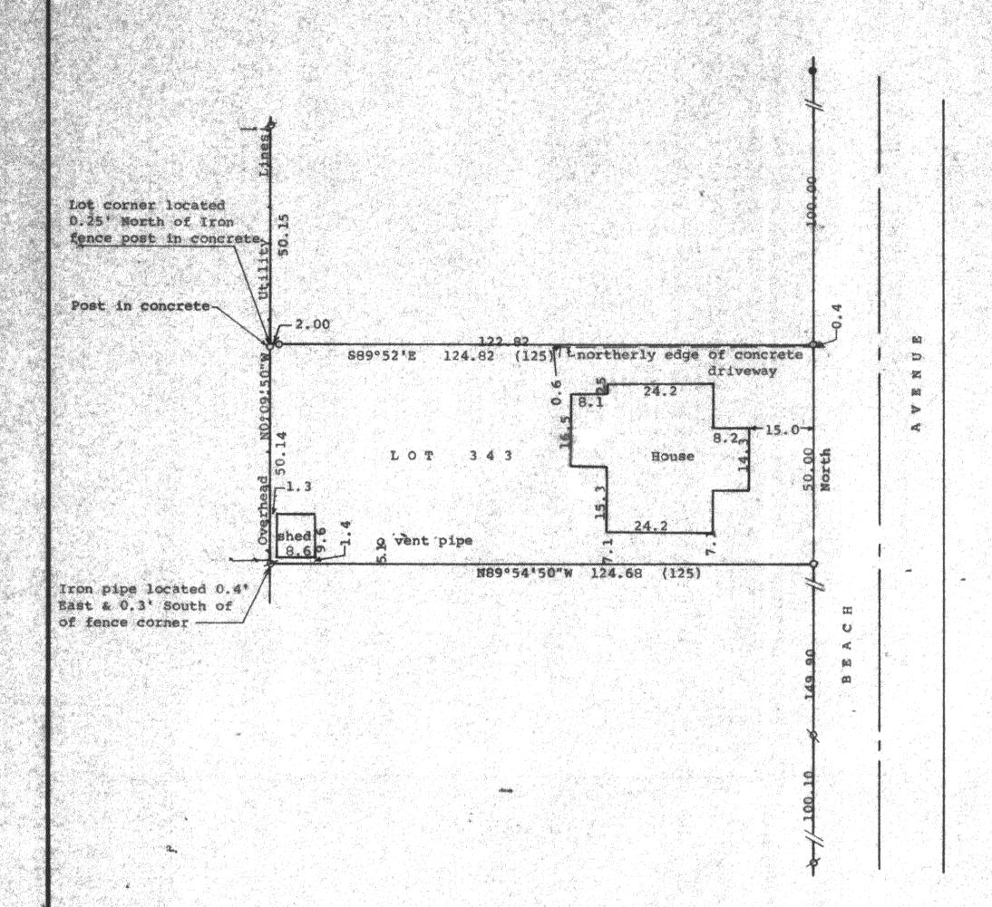
Scale - 1" = 20'  $\emptyset = 3/4$ " Iron Pipe Pound ●= 5/8" Iron Rod Found Q = 14" Iron Pipe Found O = 1" X 24" Iron Pipe Set (0.00) mecorded distance Bearings referenced to the west line of Beach Street with the assumed bearing of North Survey ordered by: Matt Drefs 121 South 6th Street Delavan, WI 53115
