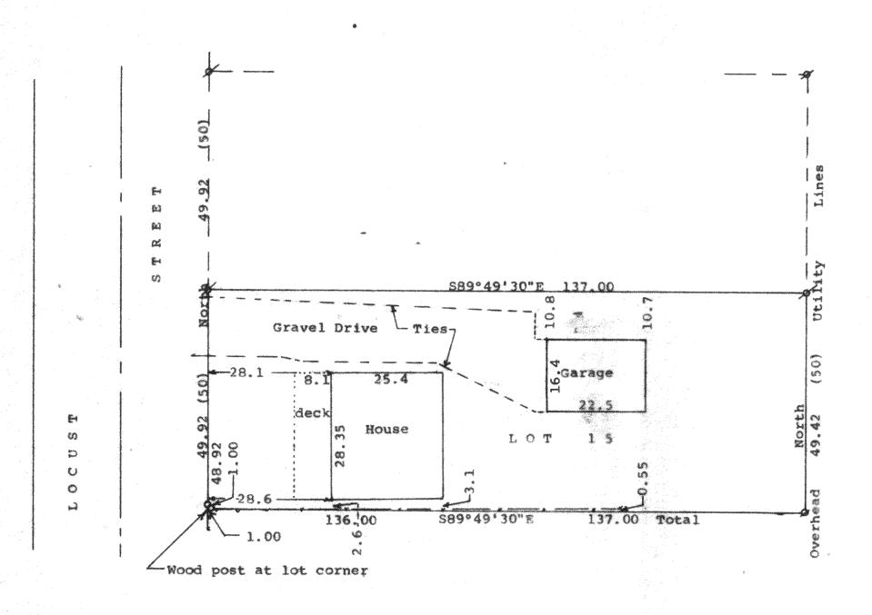
Scale - 1" = 20" $\beta = 3/4$ " Iron Pipe Found 0 = 1" X 24" Iron Pipe Set - = Fence Line (0.00) = recorded distance
