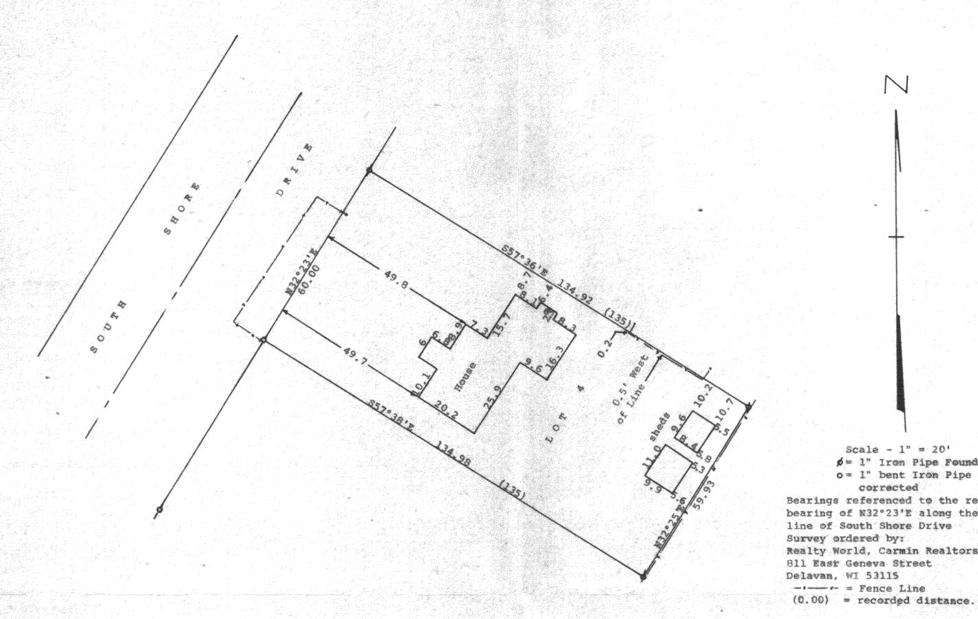
Scale - 1" = 20' ø = 1" Iron Pipe Found o = 1" bent Iron Pipe Found and corrected Bearings referenced to the recorded bearing of N32°23'E along the southeast line of South Shore Drive Survey ordered by: Realty World, Carmin Realtors 811 East Geneva Street
