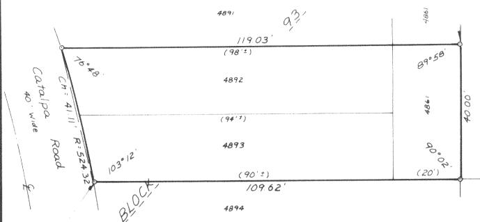
set iron nine 3' east of corner on line, tree stump at corner.
