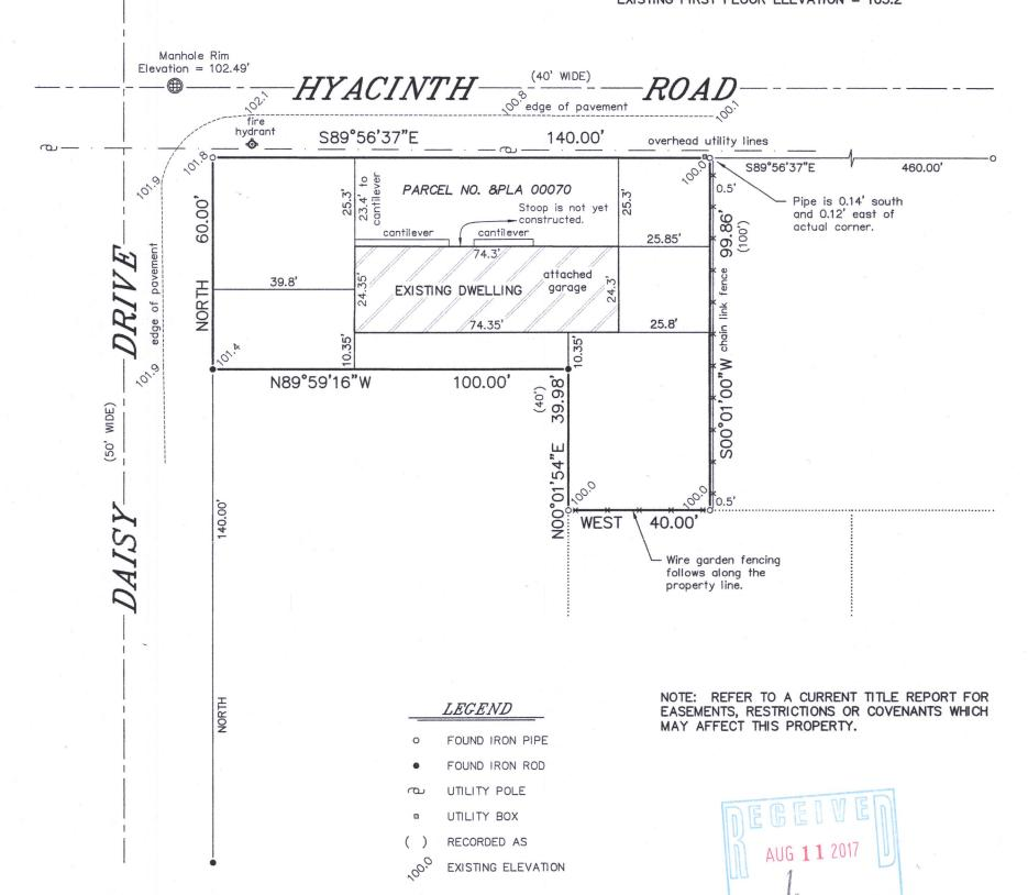
BEARINGS HEREON RELATE TO THE WEST LINE OF BLOCK 6 OF PELL LAKE ADDITION. ASSUMED BEARING OF NORTH.
