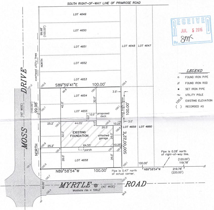
NOTE: THE PURPOSE OF THIS SURVEY IS TO SHOW THE EXISTING FOUNDATION AND ITS PROXIMITY TO THE PROPERTY LINES. ALL OTHER PROPERTY DETAILS ARE FROM PREVIOUS SURVEY WORK PERFORMED BY THIS OFFICE AND WERE NOT RE-VERIFIED AS PART OF THIS SURVEY.
