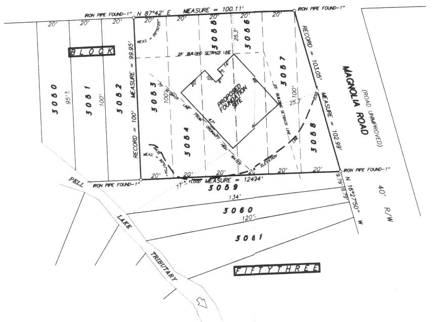
NOTE: BASE FLOOD ELEVATION (858.7') DETERMINED FROM FLOOD INSURANCE RATE MAP, COMMUNITY-PANEL NUMBER 550462 0135 B
