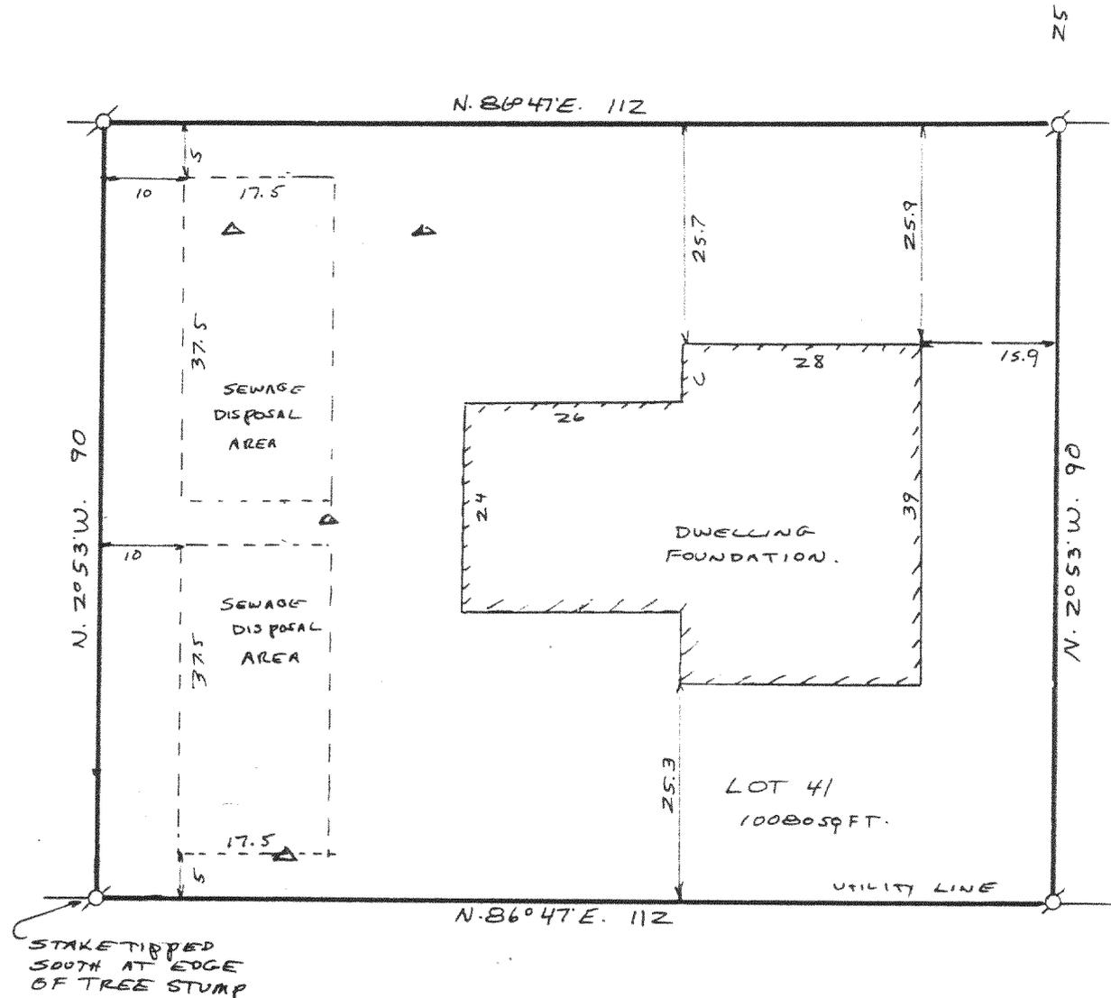
I have surveyed the above-described property, and the map hereon is a true representation thereof and shows the size and location of the property, its exterior boundaries, the location and dimensions of all visible structures thereon, fences, apparent easements and roadways and visible encroachments, if any.
