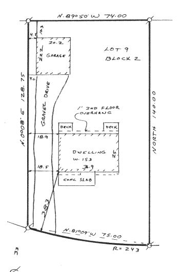
I have surveyed the above-described property, and the map hereon is a true representation thereof and shows the size and location of the property, its exterior boundaries, the location and dimensions of all visible structures thereon, fences, apparent easements and readways and visible encroachments, if any,
