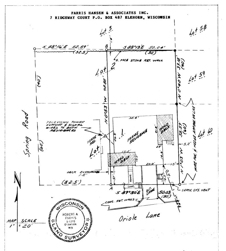
Bearing basis - line A - B between pipes found was assumed to bear N  $0^{\circ}$  53' W
