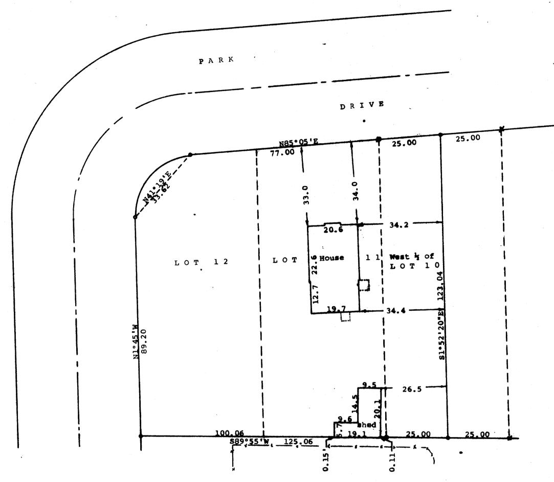
Scale -1" = 20B= Pose Pin Found • = Posey Pin Found and 3/4" X 24" Iron Pipe Set • = 3/4" % 24" Iron Pipe x= Rust mark found of Posey Pin. Spike left
