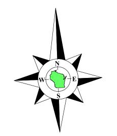
Bearings referenced to the East line of Lot 1 of Certified Survey Map No. 1926, recorded as S0°31'33"W, which produces a bearing of S89°26'49"E on the South line of the Northeast 1/4 of Section 17-1-17. A rotation of 1°50'52" from the Wisconsin State Plane Coordinate System, South Zone, (NAD-27).
