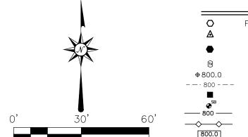
FOUND 3/4 REBAR" OR NOTED CONTROL POINT BENCHMARK SET 0.75" O.D. X 18" REBAR WEIGHING 1.502 LBS/FT. TV PED EXISTING SPOT GRADE
