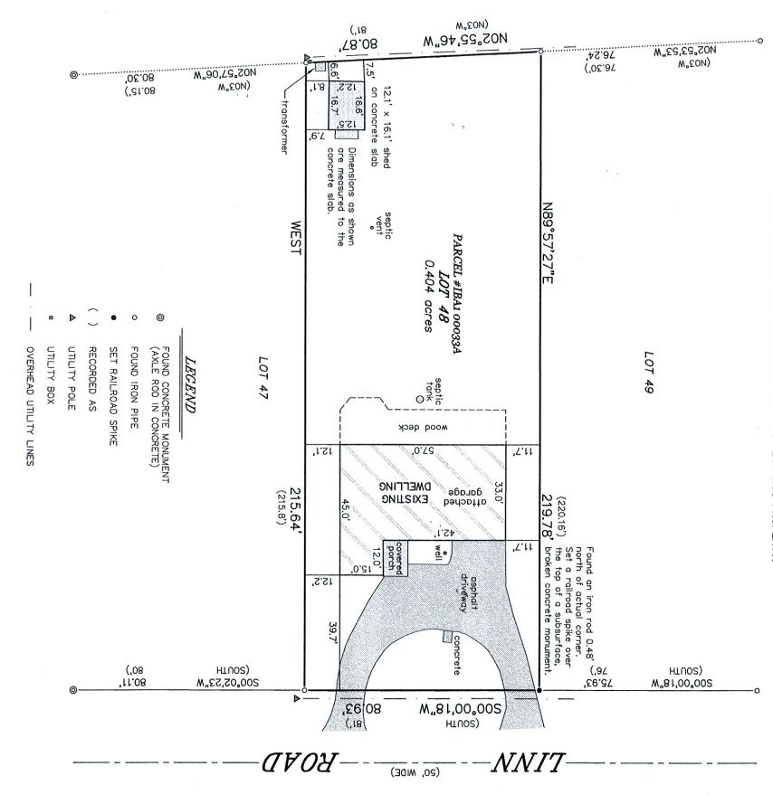
FY THAT I HAVE SURVEYED THE ABOVE RETTY AND THAT THE ABOVE MAP IS A CORRECT THEREOF AND SHOWS THE SIZE AND LOCATION TY, ITS EXTERIOR BOUNDARIES, THE LOCATION STRUCTURES AND DIMENSIONS OF ALL SINGS THEREON, BOUNDARY FENCES, APPARENT DWAYS AND ENCROACHMENTS, IF ANY."
