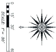
BEARINGS HEREON RELATE TO THE SOUTH LINE OF LOT 48 OF "THE BIRCHES FIRST ADDITION". ASSUMED BEARING OF WEST.
