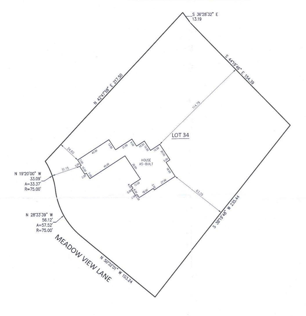
Basis of Bearing of this plat: The US State Plane Coordinate System South Zone, NAD 83. WISCORS.
