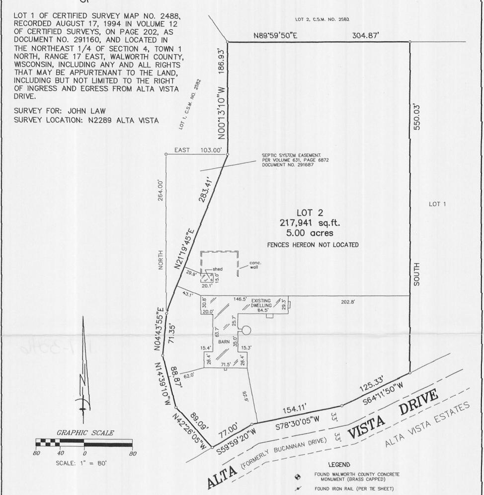
BEARINGS HEREON RELATE TO THE EAST LINE OF THE NORTHEAST 1/4 OF SECTION 4-1-17, ASSUMED BEARING SOUTH.
