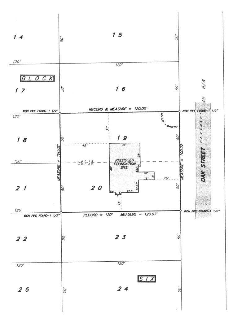
NOTE: PROPOSED FOUNDATION FIELD STAKED TRUE SIZE. CONTRACTOR TO VERIFY LOCATION AND DIMENSIONS PRIOR TO CONSTRUCTION.
