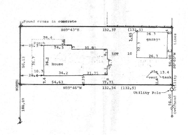
Scale -1" = 20"■ = 3/4" Dia. Iron Pipe Found o = ½" Dia. Iron Pipe Pound **%** = 3/4" x24" Iron Pipe Set • = ½"x24" Iron Pipe Set
