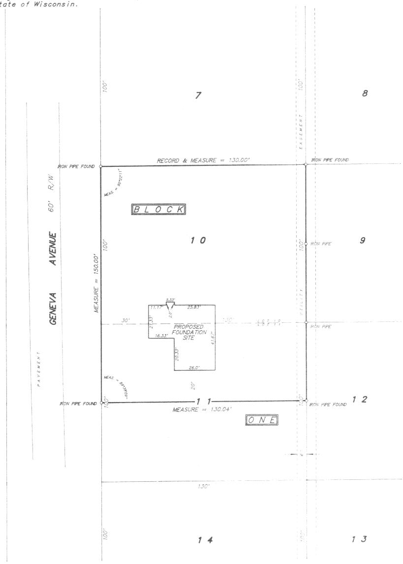
NOTE: PROPOSED FOUNDATION FIELD STAKED TRUE SIZE. CONTRACTOR TO VERIFY LOCATION AND DIMENSIONS PRIOR TO CONSTRUCTION.
