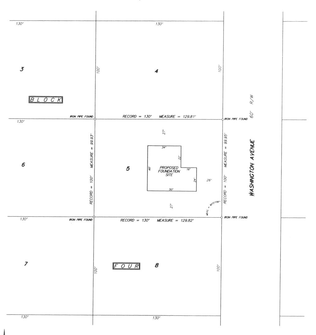
NOTE: PROPOSED FOUNDATION FIELD STAKED TRUE SIZE. CONTRACTOR TO VERIFY LOCATION AND DIMENSIONS PRIOR TO CONSTRUCTION.
