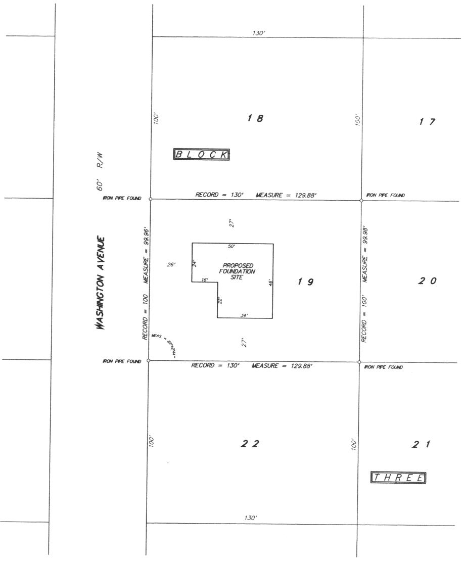
NOTE: PROPOSED FOUNDATION FIELD STAKED TRUE SIZE. CONTRACTOR TO VERIFY LOCATION AND DIMENSIONS PRIOR TO CONSTRUCTION.
