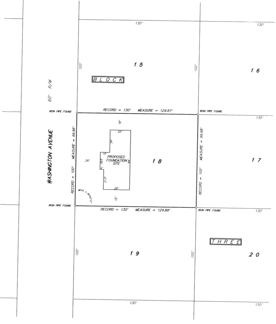
NOTE: PROPOSED FOUNDATION FIELD STAKED TRUE SIZE. CONTRACTOR TO VERIFY LOCATION AND DIMENSIONS PRIOR TO CONSTRUCTION.
