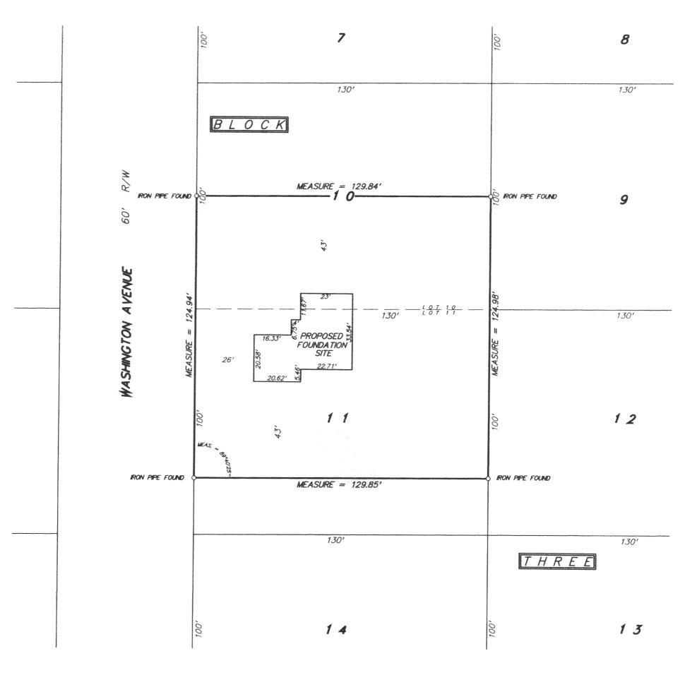
NOTE: PROPOSED FOUNDATION FIELD STAKED TRUE SIZE. CONTRACTOR TO VERIFY LOCATION AND DIMENSIONS PRIOR TO CONSTRUCTION.
