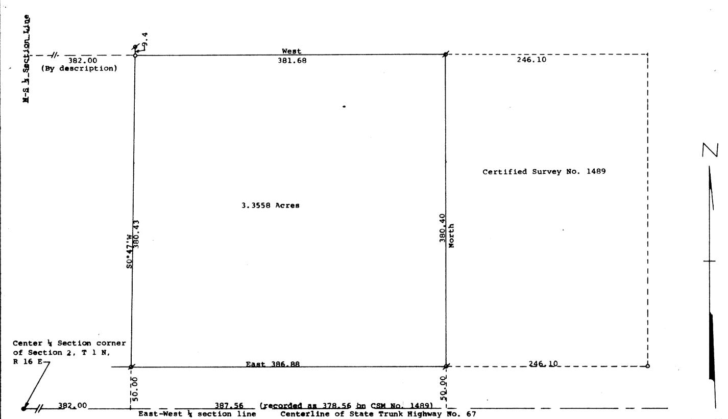
Scale - 1" = 60 Feet #= 14" Iron Pipe Found o = 1" X 24" Iron Pipe Set • = County conc. marker found Bearings referenced to the assumed bearing of East along the south line of the NE's of Section 1, TlN, R16E Owner: Geryl & Helen Blakeley Highway 67 Williams Bay, WI 53191
