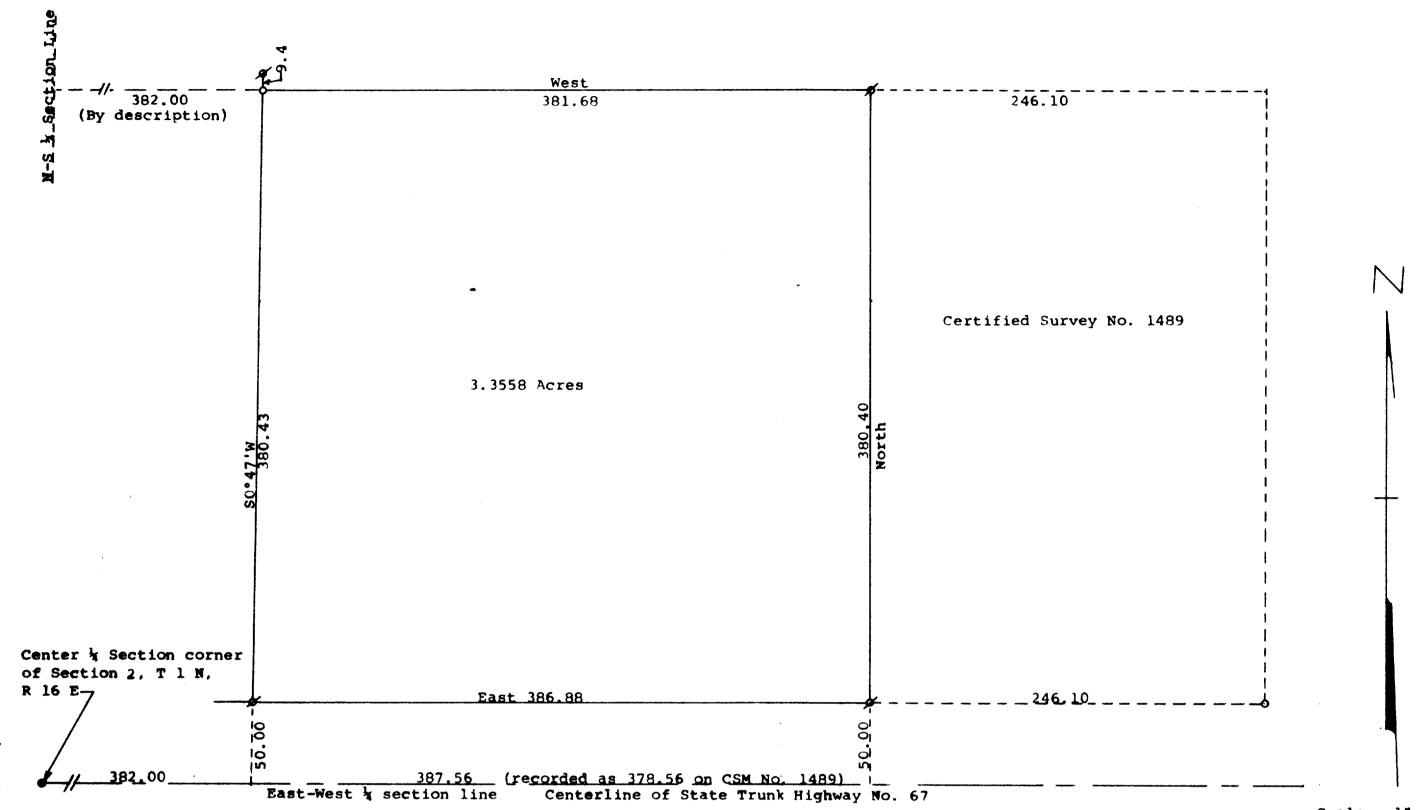
Scale - 1" = 60 Feet #= 14" Iron Pine Found O = 1" X 24" Iron Pipe Set = County conc. marker found Bearings referenced to the assumed bearing of East along the south lin of the NE% of Section 1, TlN, R16E Owner: Geryl & Helen Blakeley Highway 67 Williams Bay, WI 53191
