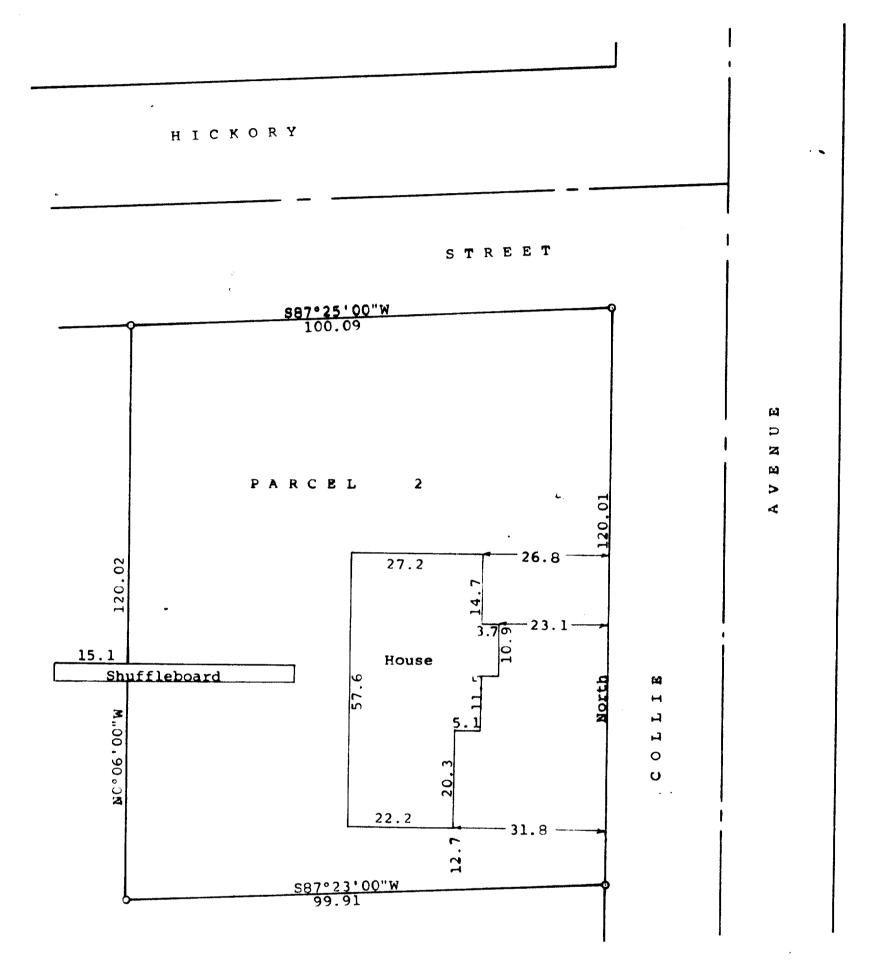
Scale -1" = 20'O = 1" Iron Pipe Found Bearings are referenced to the west line of Collie Avenue with the assumed bearing of North.
