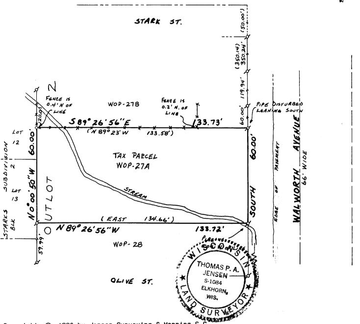
Copyright © 1990 by Jensen Surveying & Mapping S.C All rights reserved. No part of this survey plat may be reproduced or transmitted in any form by any means - graphic, electronic, or mechanical, including photocopying, tracing, or information storage and retrieval systems - without permission in writing from Thomas P.A. Jensen.
