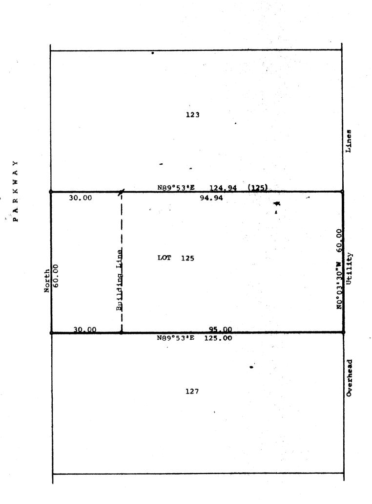
Scale - 1" = 20\* o = 1" Iron Pipe Found #= 4" Iron Pipe Found Bearings referenced to the east line of Lincoln Parkway with the assumed bearing - North Survey ordered by: Marilyn Javorski 8355 South Latrobe Burbank, IL 60459
