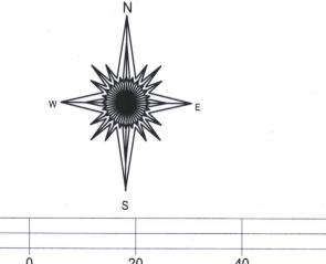
BASIS OF BEARING OF THIS PLAT THE US STATE PLANE COORDINATE SYSTEM SOUTH ZONE NAD 83 WISCORS.
