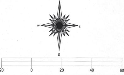
BASIS OF BEARING OF THIS PLAT: THE EAST LINE OF BAY VIEW RD. WAS ASSUMED TO BEAR N 18°45' W AS SHOWN ON OTHER SURVEYS OF RECORD.
