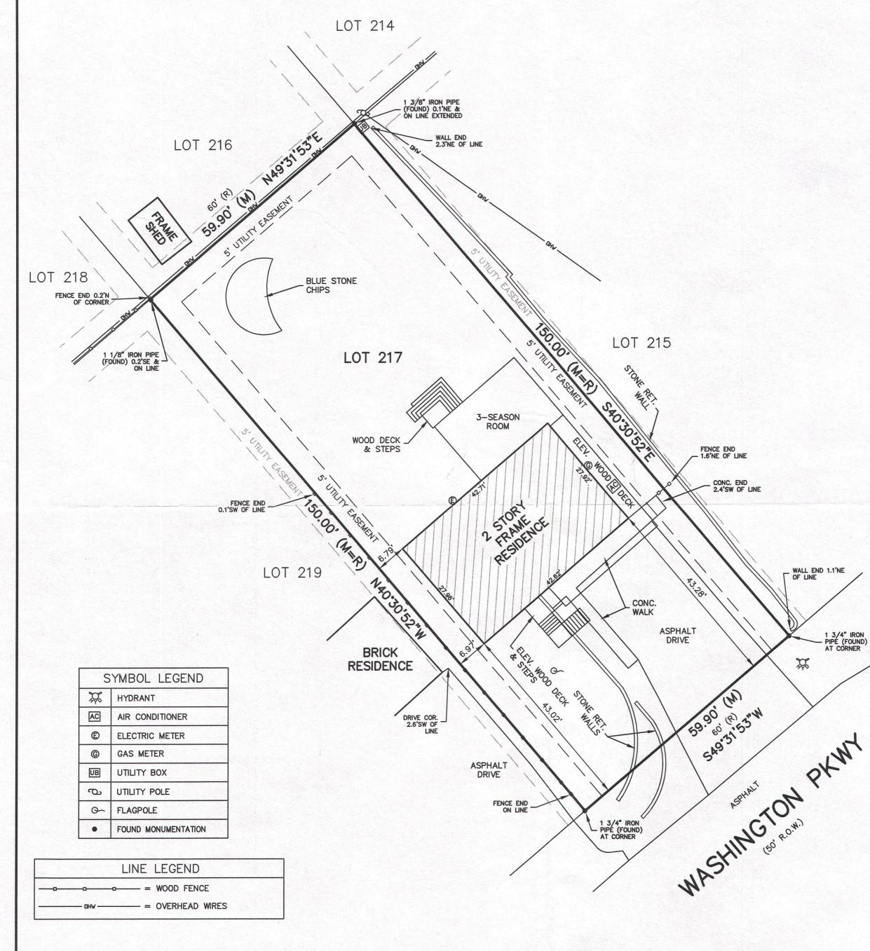
NOTE: BUILDING TIE DIMENSIONS SHOULD NOT BE USED TO DETERMINE LOT LINE LOCATIONS. REFER TO ACTUAL LOT CORNERS AND REPORT ANY DIFFERENCES TO THE SURVEYOR IMMEDIATELY.
