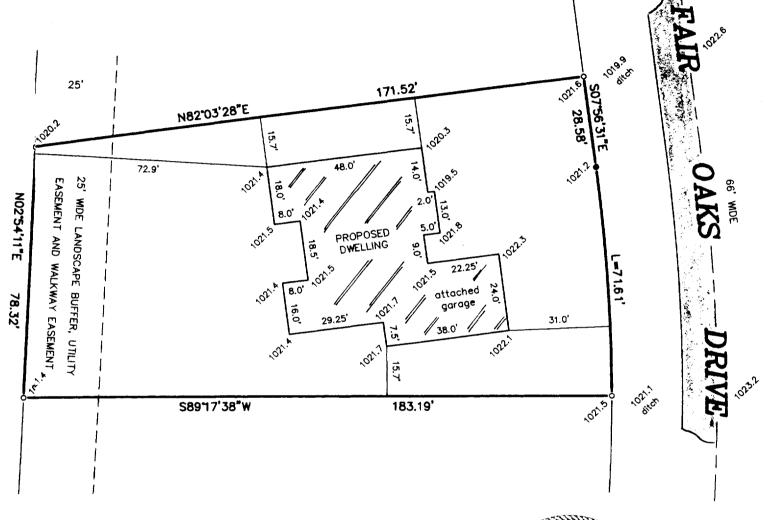
PROPOSED DWELLING W.S STAKED ON ACTUAL CORNERS WITH SEVEN FOOT CONTROL ON THENORTHERLY HOUSE LINE. THE CONTRACTOR WILL BE RESPONSIBLE D FIELD VERIFY ALL STAKES FOR LOCATION AND DIMENSION PRIOR O CONSTRUCTION. THIS OFFICE SHOULD BE NOTIFIED IMMEDIATELY II ANY DISCREPANCIES OCCUR.
