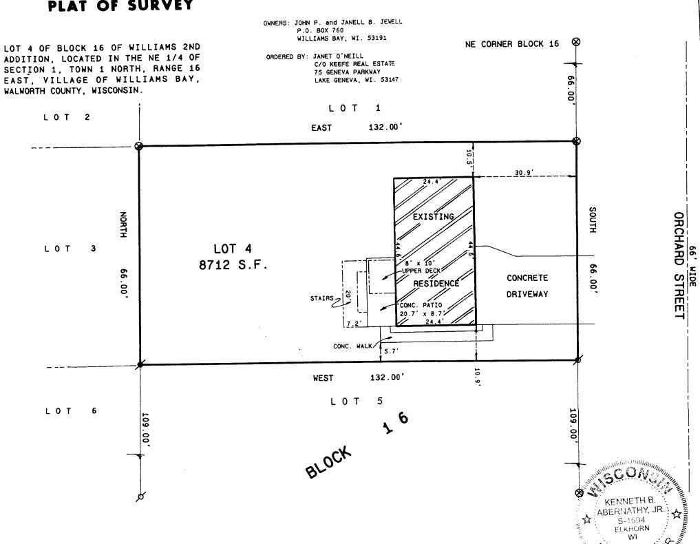
SCALE: 1"= 20 FEET Legend FOUND IRON PIPE FOUND IRON ROD FOUND BRASS CAPPED MONUMENT FOUND CONCRETE MONUMENT CHISEL CUT IN CONCRETE SET IRON ROD, 24" LONG, WEIGHING 1.5 LBS./LINEAL FT., 3/4" DIA. SET IRON ROD, 30" LONG, WEIGHING 4.5 LBS./LINEAL FT., 1-11/16" DIA. RECORDED AS DIMENSION -x-x- EXISTING FENCE "I hereby certify that | have surveyed the above described property and that the above map is a true representation thereof and shows the size and location of the property, its
