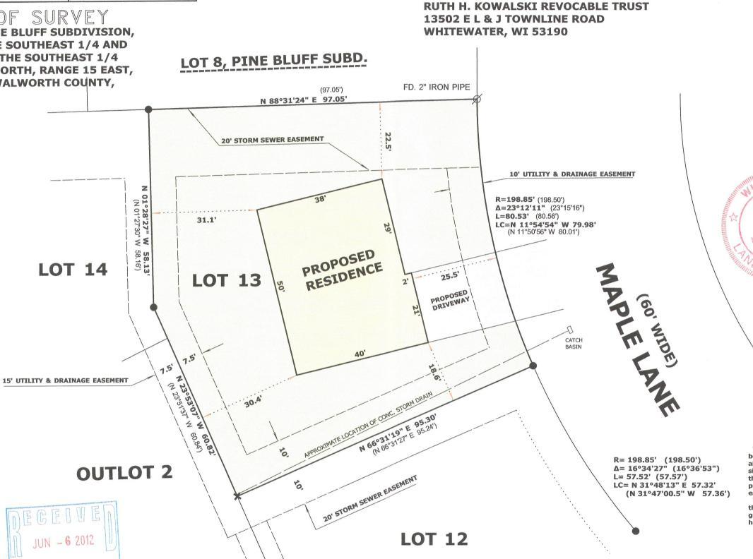
CONS MARKL MIRITZ WHITEWATER, WI **LEGEND FOUND IRON PIPE** FOUND CUT CROSS ON CONCRETE DRAIN PIPE SET IRON ROD, 18" LONG, WEIGHING 1.5 LBS./LINEAL FT., 3/4" DIA. RECORDED AS DIMENSION SCALE: 1 INCH = 20 FEET "I hereby certify that the above described property has
