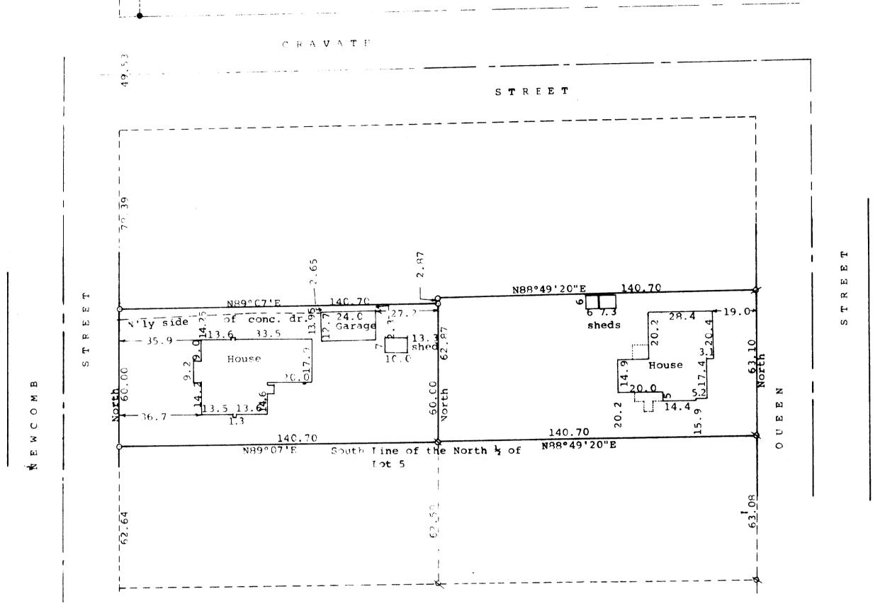
Scale - 1" = 30'•= 15" Iron Rod Found 英= 1" Iron Pipe Set ○ = 3/4" Iron Pipe Set Bearings referenced to the east line of Newcomb Street with the assumed bearing of North Survey ordered by: Dean Hollinger 235 North Newcomb Street Whitewater. WI 53190 % = 1" Iron Pipe Found
