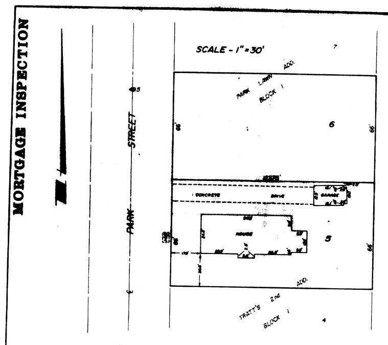
NOTE: Lot dimensions are shown as recorded on the original plat. These dimensions were not necessarily verified in the field and no lot stakes were set in the course of this inspection.
