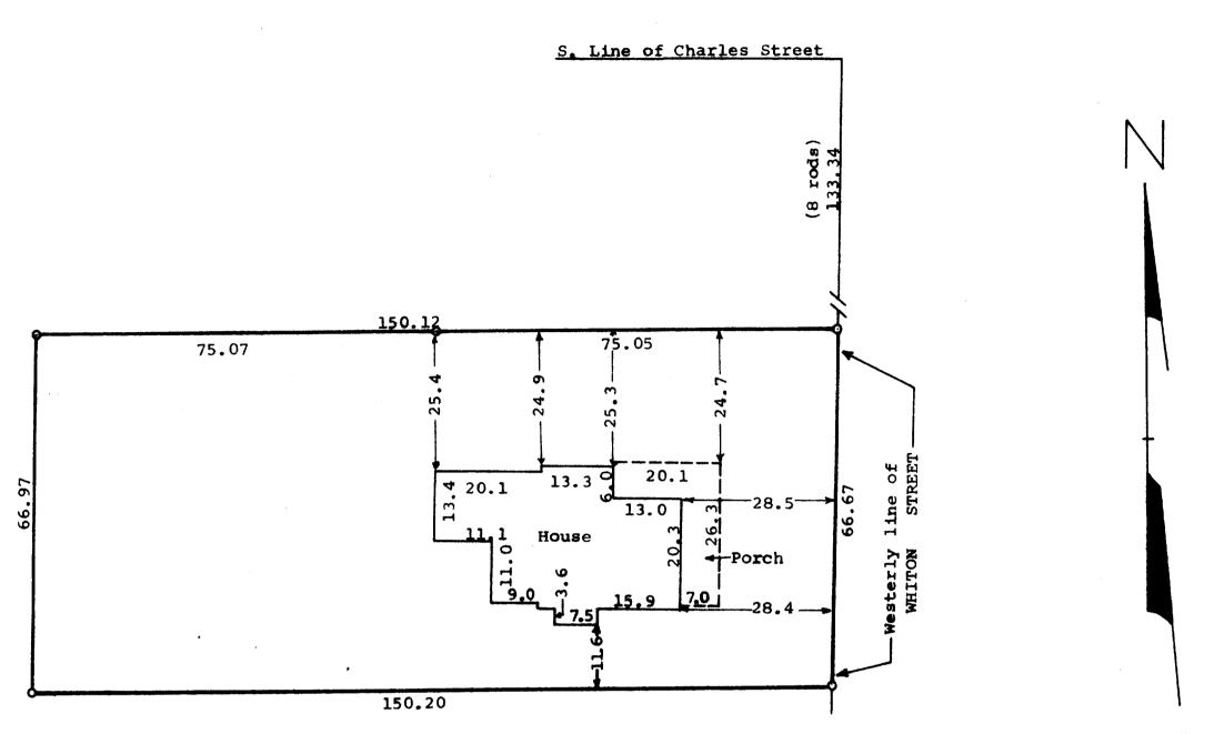
Scale -1" = 20'0 = Iron Pipe Set Note: The differences in the distances shown on the plat of survey and those in the description of the property are due to overrun in Block 3 of Birge's Addition.
