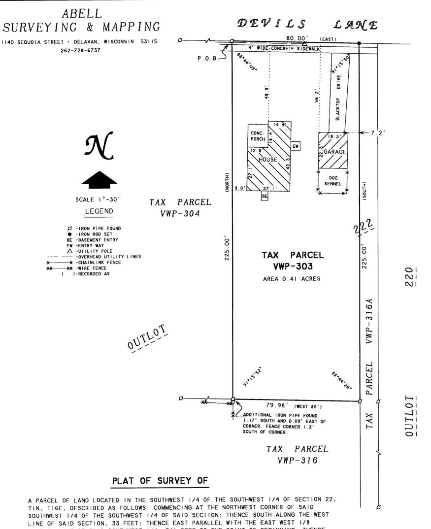
SECTION LINE OF SAID SOUTHWEST 1/4, 741 FEET TO THE POINT OF BEGINNING: THENCE CONTINUE EAST ON THE SAME LINE 80 FEET: THENCE SOUTH PARALLEL WITH THE WEST LINE OF SECTION 22. A DISTANCE OF 225 FEET: THENCE WEST 80 FEET: THENCE NORTH 225 FEET TO THE POINT OF BEGINNING. SAID PARCEL BEING A PART OF OUTLOT 222 OF THE ASSESSOR'S PLAT OF THE VILLAGE OF WALWORTH, WALWORTH COUNTY, WISCONSIN.
