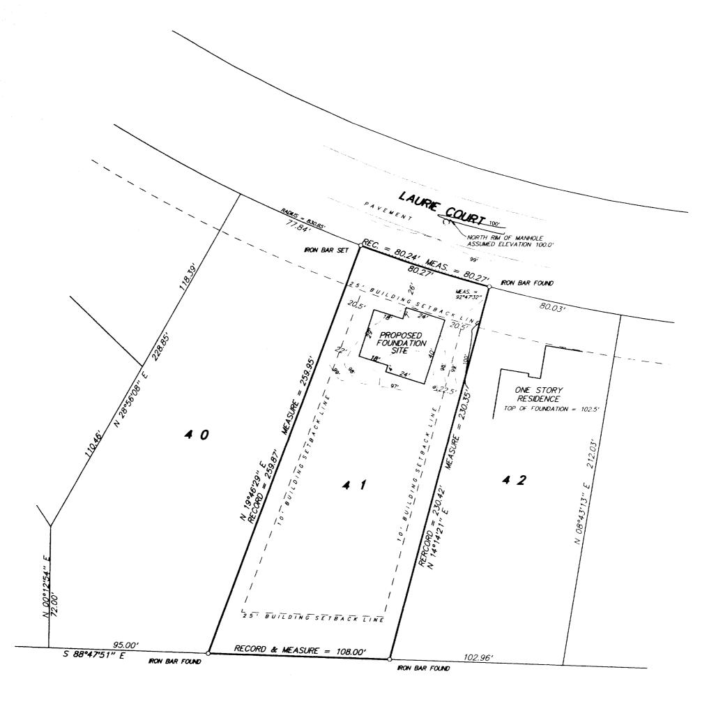
NOTE: PROPOSED FOUNDATION FIELD STAKED TRUE SIZE. CONTRACTOR TO VERIFY LOCATION AND DIMENSIONS PRIOR TO CONSTRUCTION.
