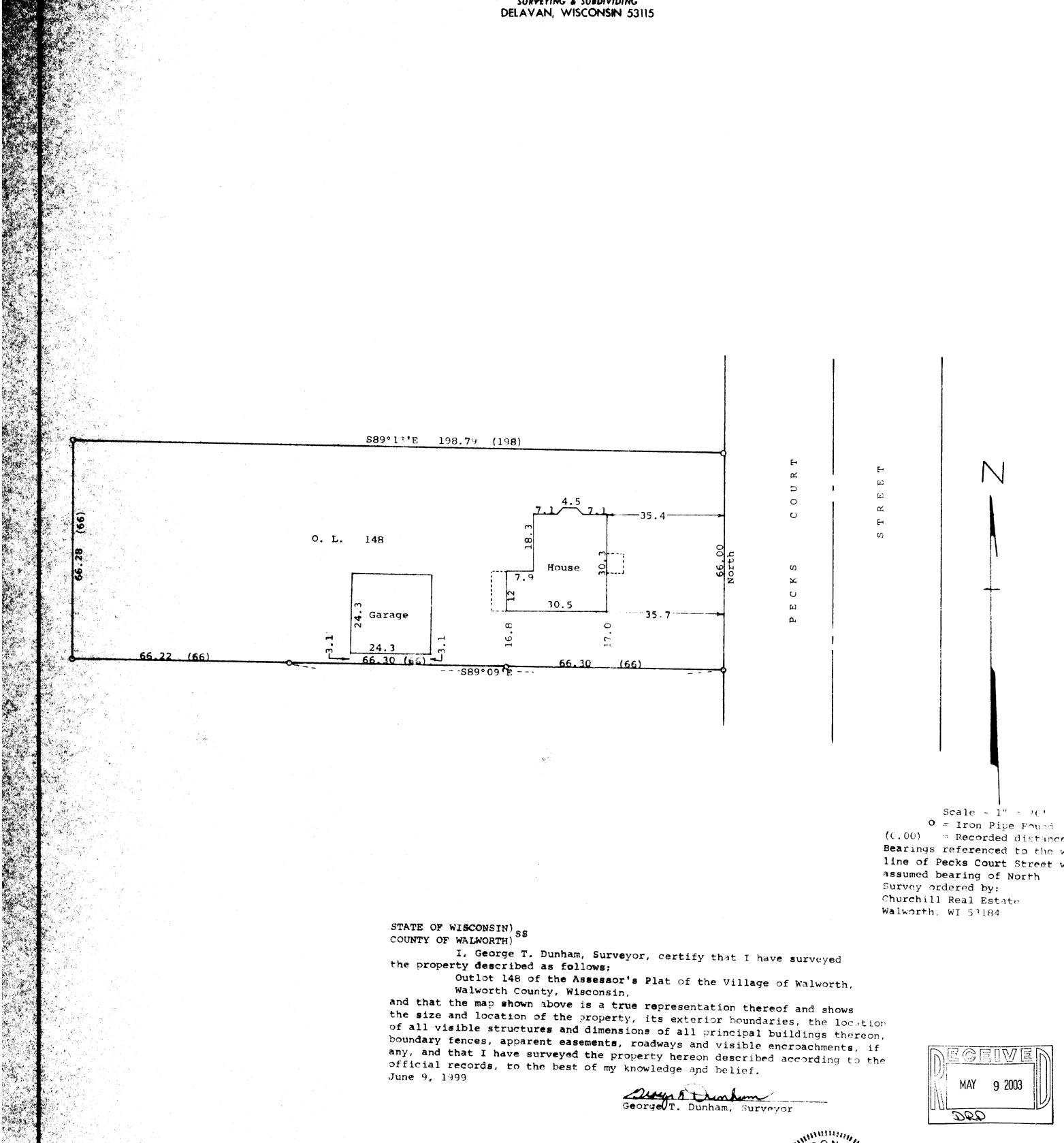
Scale - 1" = 261 O = Iron Pipe Found (0.00) = Recorded distance Bearings referenced to the west line of Pecks Court Street with the assumed bearing of North Survey ordered by: Churchill Real Estate Walworth, WI 53184
