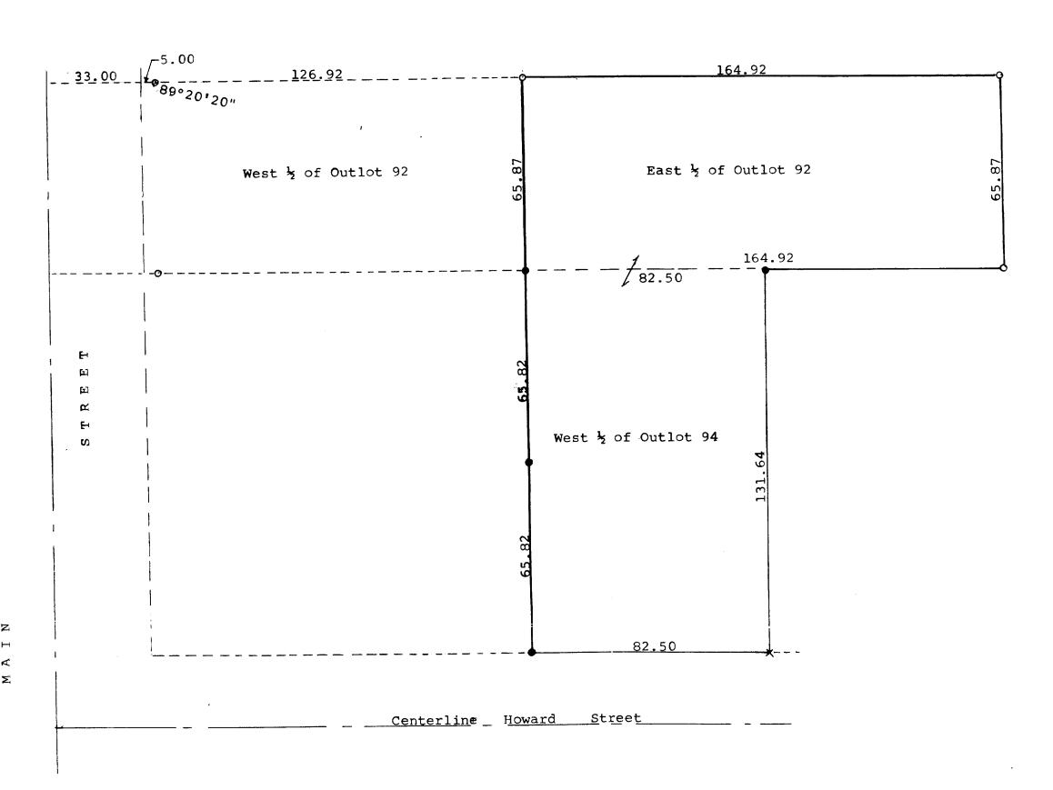
Scale - 1" = 30; O = Iron Pipe ● = Iron Rod x= Chisel Mark Survey ordered by: Jeff Dixon 114 Howard Street Walworth, WI 53184
