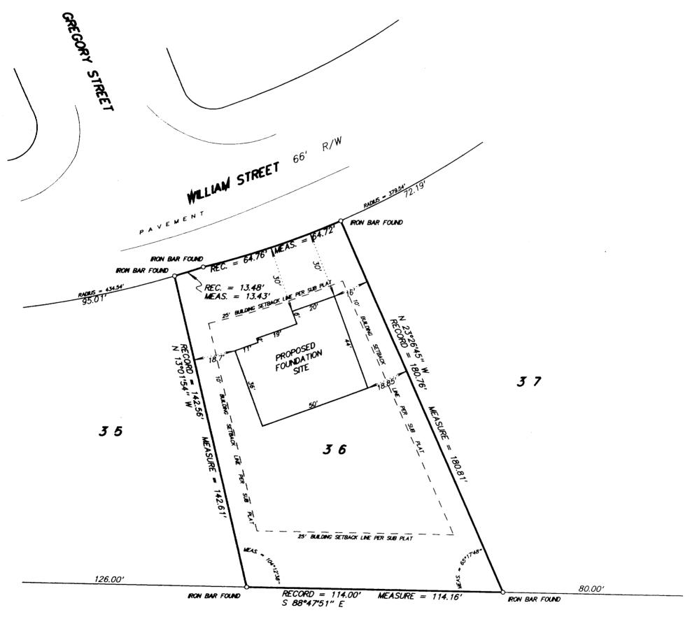
NOTE: PROPOSED FOUNDATION FIELD STAKED TRUE SIZE. CONTRACTOR TO VERIFY LOCATION AND DIMENSIONS PRIOR TO CONSTRUCTION.
