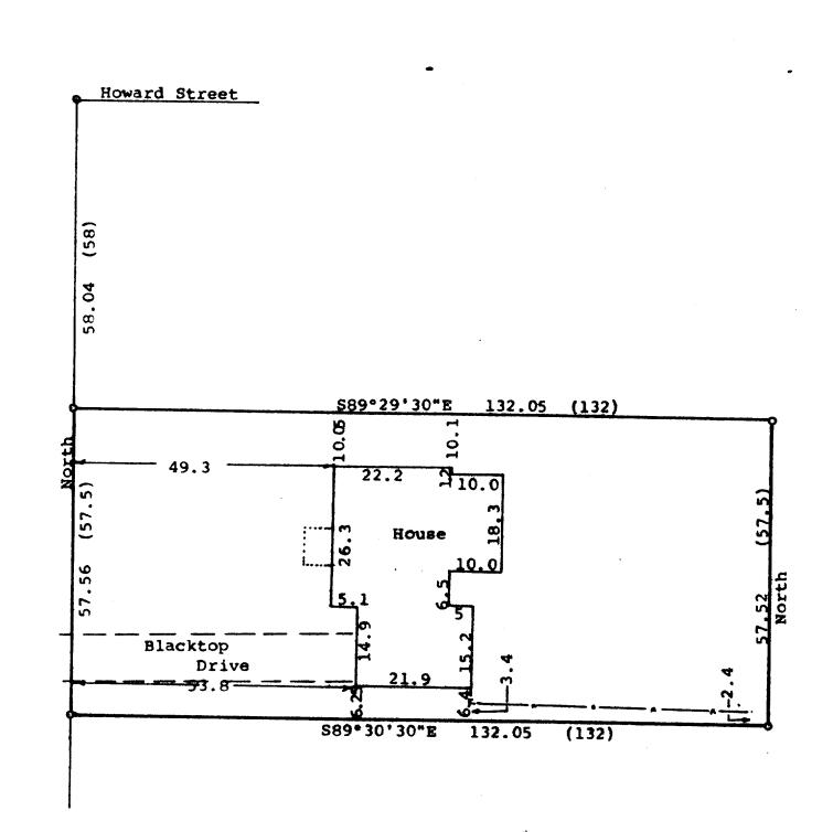
Scale - 1" = 200 = 3/4" Iron Pipe Found (0.00) = recorded distance ---- Fence Line . Bearings referenced to the east line of Pecks Court with the assumed bearing of North Survey ordered by: Churchill Real Estate 322 Park Walworth, WI 53184
