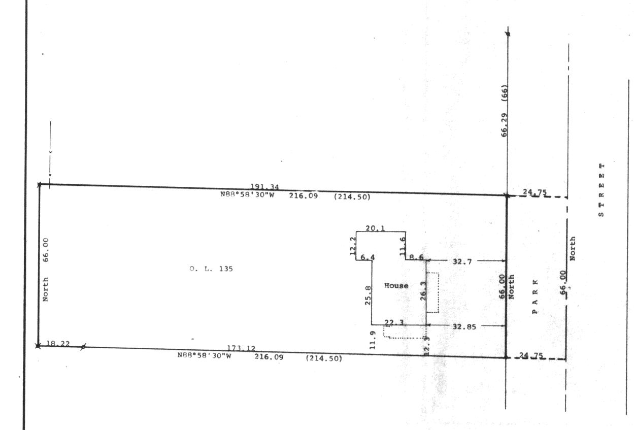
Scale - 1" = 20"• = 3/4" Iron Rod Found  $\beta = 3/4$ " Iron Pipe Found x = 1" Iron Pipe Found N = 14" Iron Pipe Found Bearings referenced to the west line of Park Street with the assumed bearing of North (0.00) = recorded distance Survey ordered by: Churchill Real Estate 322 Park Street
