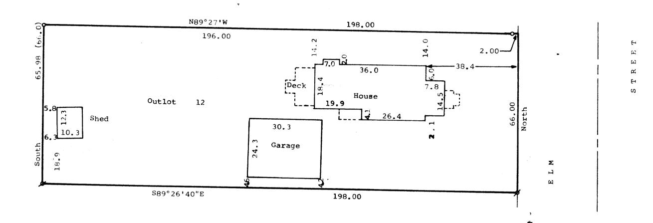
Scale - 1" = 20' O = 1" Dia. Iron Pipe Found Ø = 1"x24" Iron Pipe Set (66.0) = Recorded Distance Bearings are based on the West line of Elm Street, assumed bearing of North. Survey Ordered By: Churchill Real Estate 322 Park Street Walworth, WI 53184
