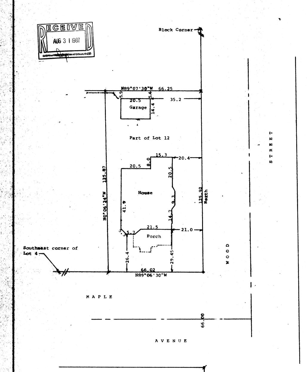
Scale - 1" = 20' # = 1%" Iron Pipe Found = 3/4" Iron Pipe Found o = 1 Iron Pipe Found x = Iron Pipe Found under sidewalk. Cross cut in concrete
