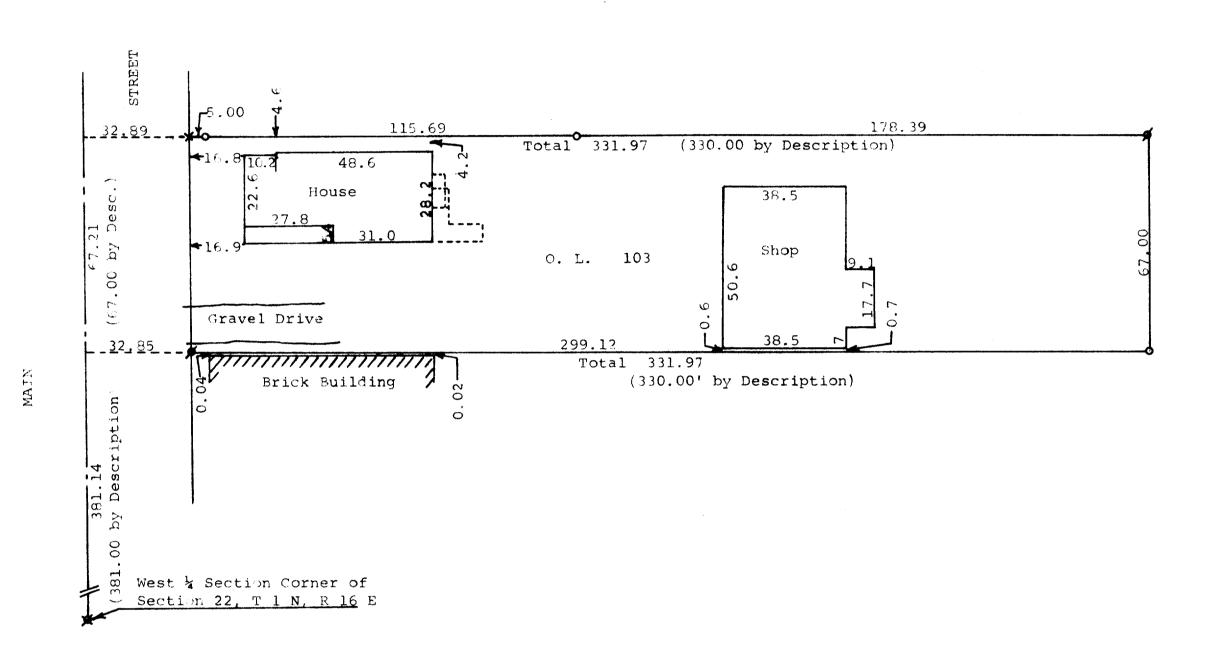
Scale - 1'' = 30'**≠** = Iron Pipe Found **X** = Metal Plate Found • = Iron Rod Found X= Cross in Conc. Found • = Iron Pipe Set
