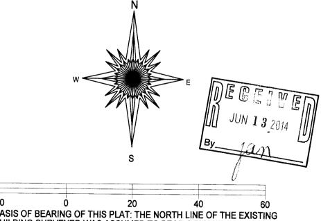
BASIS OF BEARING OF THIS PLAT: THE NORTH LINE OF THE EXISTING BUILDING SURVEYED WAS ASSUMED TO BEAR S 57°00'E AS RECORDED.
