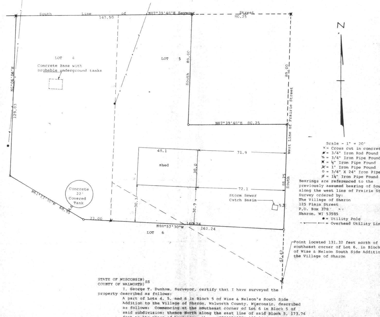
X = Cross cut in concrete # = 3/4" Iron Rod Pound  $\alpha = 3/4$ " Iron Pipe Found X = ½" Iron Pipe Found X = 1" Iron Pipe Found 0 = 3/4" X 24" Iron Pipe Set
