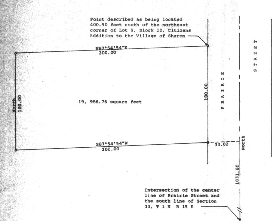
Scale - 1" = 30"• = Concrete Monument Found O = 1" X 24" Iron Pipe Set Bearings referenced to the centerline of Prairie Street with the assumed bearing of North Survey ordered by: Mikrut Realty
